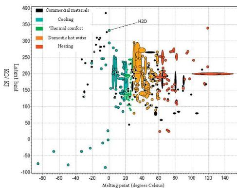
Figure 1. Relationship between melting point and latent heat for phase change materials in different applications [7].
