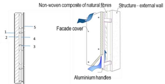
Figure 1. Left) Cross section, 1. Internal wall of 22 cm solid brick, 2. Non-woven composite of natural fibers, 3. Aluminum handles, connecting the facade covering to the inner wall, 4. Air layer, 5. Facade covering. Right) The proposed model of shell façade - Fiber composite panels with natural fibers are placed on the outer shell of the building façade as a moisture and heat retarder. There should be a space for air conditioning between the façade cover and the composite.
