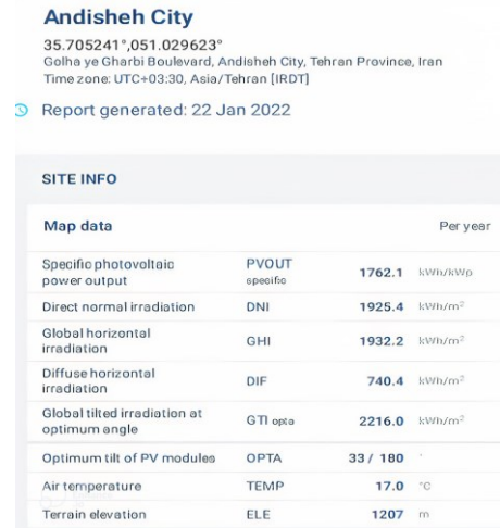
Figure 1. World Atlas of the Sun data for the new city of Andisheh
