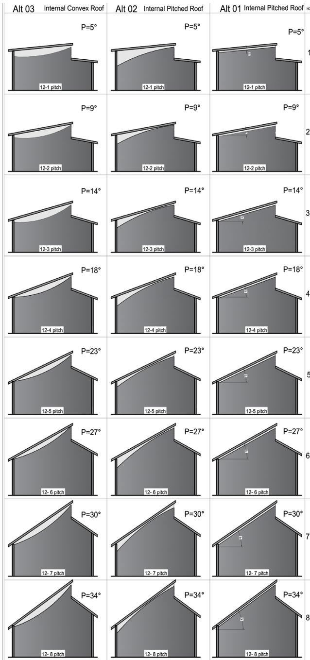
Table 1 Cross-section of test models in octagonal slope ratio
