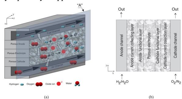
**Figure 1.** (a) Schematic illustration of a single cell of planar-type AP-SOFC, (b) cross-section of planar-type AP-SOFC representing the computational domain (detailed "A")
